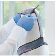
The 616B60 resin film was developed especially to support the production of exceptionally highly stable and lightweight prostheses and orthoses using lamination technology.
