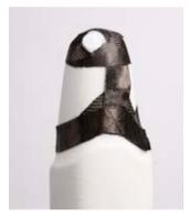
• 1-2 naps (carbon fibre cloth) for residual limb cap
