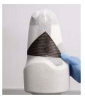
• 1 triangle (carbon fibre cloth) for medial torsion stiffening
