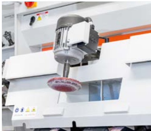
Sensor controlled extraction at the naumkeag As soon as a workpiece is processed on the naumkeag, dust extraction is activated and only the extraction ports on the naumkeag are opened for full extraction performance.
