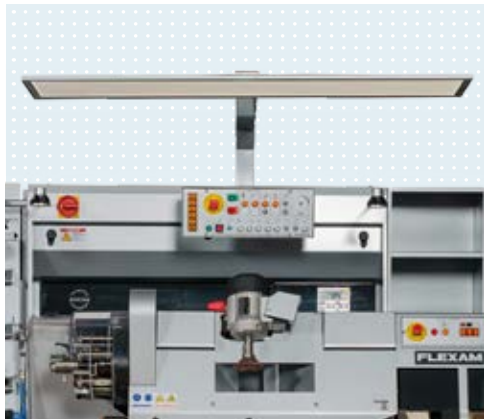
Lighting: LED flood lamp Additional LED flood lamp, supplementing the two LED spotlights for optimum illumination of the workstation.
