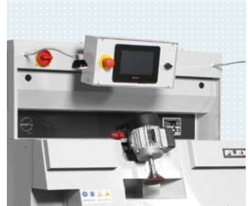
Control panel: touchscreen Individual control, personal profiles and remote maintenance.
