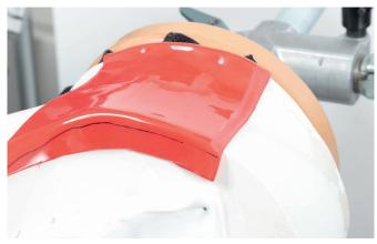
Mark the edge to be bevelled. Bevel the edge at the socket router. Place the material on the plaster model.
