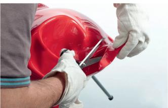
Using scissors, cut off any excess material at the seams. This prevents the weight of the excess material from stretching the areas.
