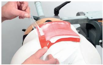
Remove the adhesive tape immediately after the parting agent has been applied.
