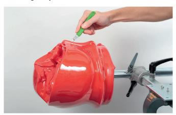
Cut open the prosthetic socket in the middle above the Neoprene® cellular rubber tape. Do not cut into the tab while doing so.
