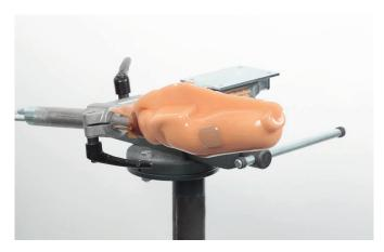
Seal the area around the vacuum tube with sealing tape (e.g. made from Vulkollan®).
