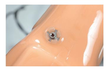
Press the lamination disk into the material until the material that has been pressed through is flush with the surrounding material.
