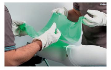
Lift the heated material at its 4 corners and drape it over the plaster model.
