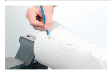
Mark the flexible proximal section on the plaster model. Select the suitable material thickness.
