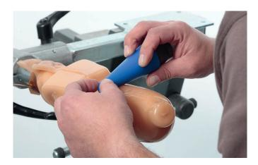
Smooth the seam with a silicone sanding cone.
