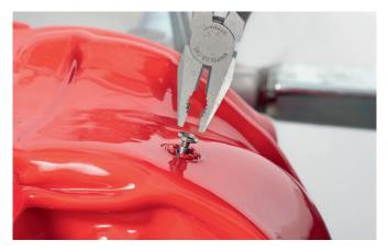
When the material is soft enough, press the lamination disks into the material. The material is pressed through the slotted holes in the lamination disk.
