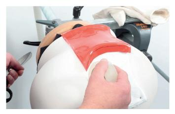
Mask the part of the tab that is to be welded to the prosthetic socket with PE adhesive tape.
