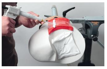
Apply a silicone-based parting agent (e.g. BetaSil, Impresil or silicone bonding agent) to the material.
