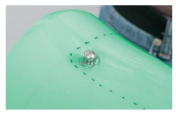
When the material is soft enough, press the lamination disks into the material until the material extrudes slightly from the slotted holes in the lamination disk.
