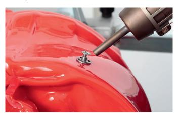
Screw a screw into each lamination disc until the thread is completely filled. This prevents the material from entering the thread.
