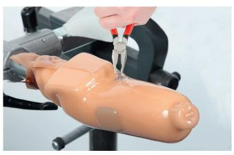
When the material is soft enough, press the lamination disks into the material. The material is pressed through the slotted holes in the lamination disk.
