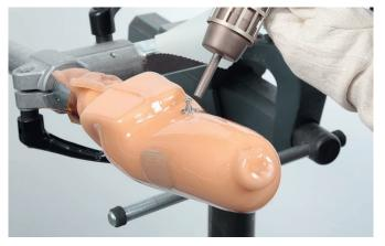
Heat the lamination disk and the surrounding material with the hot air gun.
