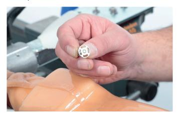
Screw a screw into each lamination disc until the thread is completely filled. This prevents the material from entering the thread.
