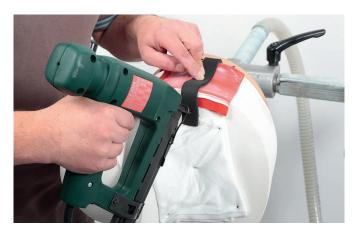
Cut a strip of Neoprene® cellular rubber tape to size and place it where the inner socket is to be opened. Attach the Neoprene® cellular rubber tape with a stapler.
