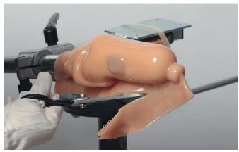
Using scissors, cut off any excess material at the seam. This prevents the weight of the excess material from stretching the area around the seam.
