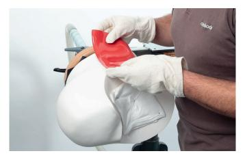
Lift the heated material and place it on the plaster model.
