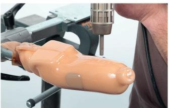
Using a scalpel, cut off any excess material flush with the seam.
