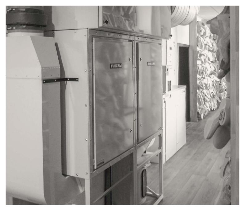
The V80 dust extractor is available as both a centralised and decentralised extraction system.
