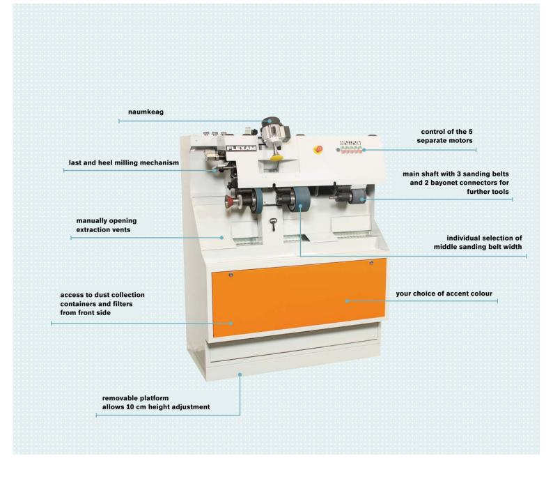
This compact grinding and milling machine with a naumkeag and integrated dust extractor is an optimal stand-alone and starter solution for processing lasts and inserts and for the basic construction of orthopaedic footwear.
